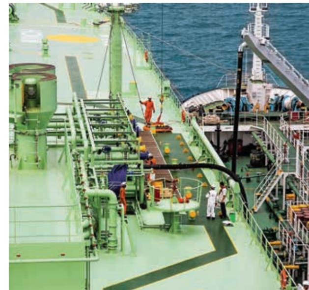
Bunker operations underway onboard VLGC BW Volans
